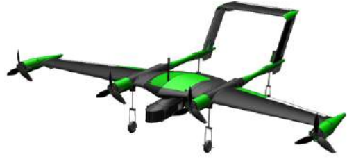
Figure 5: STOL configuration of this RPV model.
