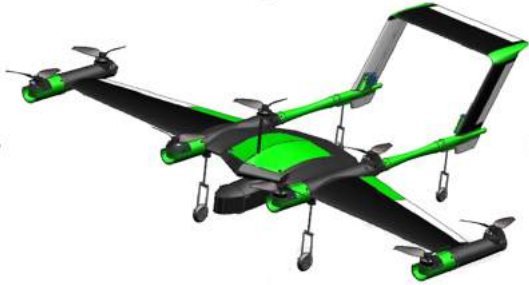
Figure 8: VTOL configuration of this RPV model.
