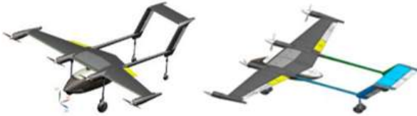
Figure 2: 3D CAD model of the 1-by-10 Flexcraft scaled version [10].
