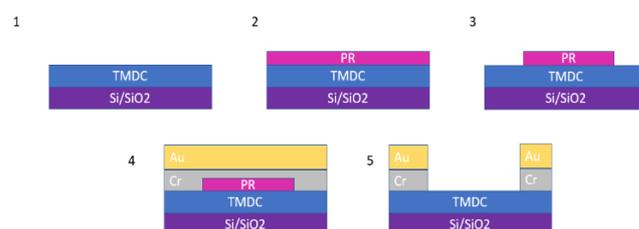
Figure 7 - Schematics for the cleanroom fabrication steps: 1. CVD grown MoSe<sub>2</sub> on Si/SiO<sub>2</sub> 2. Photoresist spin coating 3. Photoresist patterning through direct write laser 4. Metal contact deposition. The metal contact is a stack consisting on 20 nm of gold stack on 3 nm Cr, for adhesion
