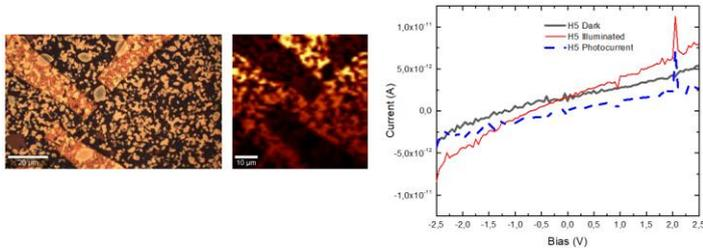
Figure 8 - Device H5 exhibits photocurrent when illuminated with a white LED. The quality of the film in between the contacts was investigated under Raman
