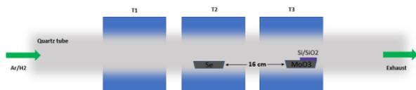
Figure 3 - CVD system schematic and crucible position example. In this image the crucibles are spaced
