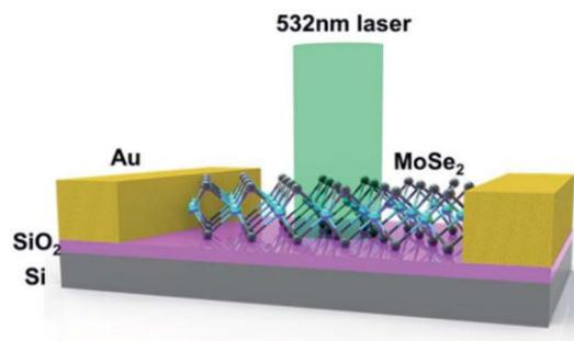
Figure 2 - Schematic of a MoSe<sub>2</sub>-based photodetector with gold contacts<sup>9</sup>.
