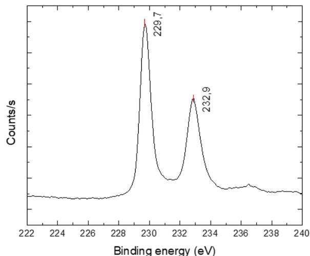
Figure 6 - XPS measurements performed on sample M07, 4 months after production
