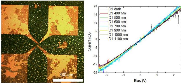
Figure 9 - Optical bandgap of the sample measured on device D1 using a light source coupled with a monochromator
