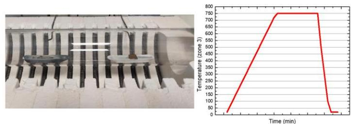
Figure 4 - Precursor boat and substrate configuration (left) and temperature profile during procedure (right)
