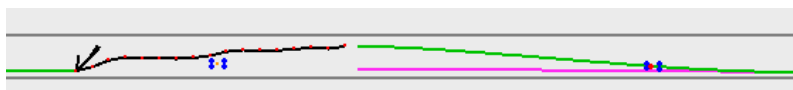
Figure 3.7: RRT path retracing, with the new trajectory in black, with nodes in red. Notice how the K1999 then creates a return path to the optimal trajectory, only at the end of the retraced line.
