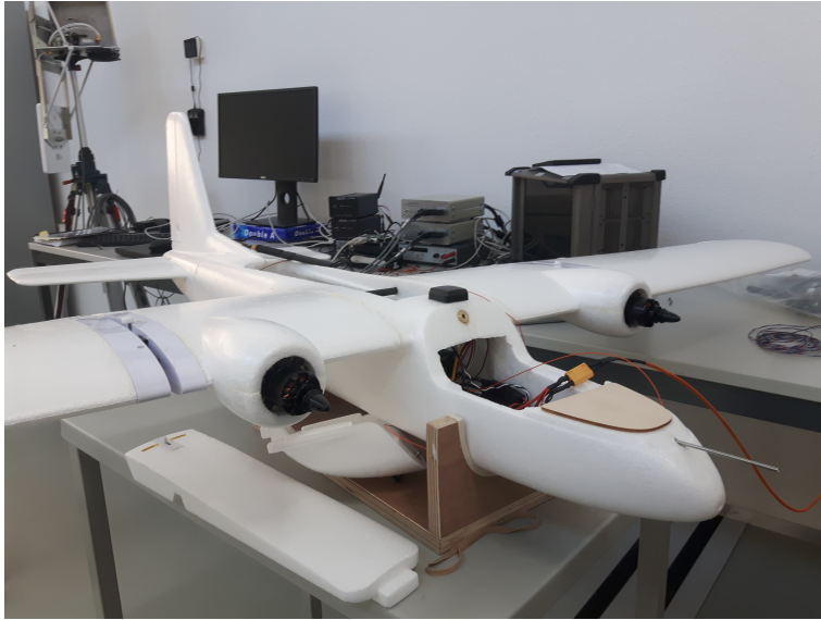
Figure 6.1: The MyTwinDream UAV with its propeller blades removed.
