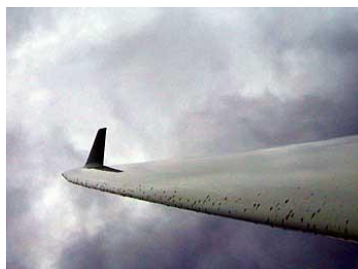
Figure 2.5: Leading edge contamination [32].
