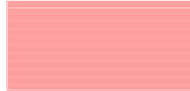
Figure 20: Stress Optimization for Straight fibers - Optimal Solution for the plate without a hole: w_{time} = 1 and w_{strain} = 0
