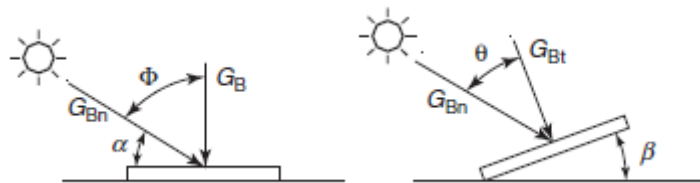
Figure 37 - Beam irradiance on horizontal and tilted surfaces. Source: [24]
