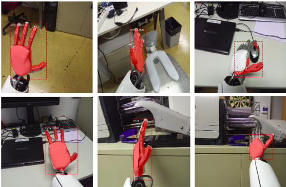
Figure 8: Visualization of the predicted masks, bounding boxes and class scores, for 6 images of the real test dataset.
