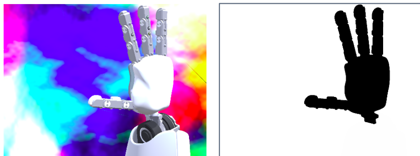
Figure 3.6: Example of an image generated in the simulator (left) and its corresponding groundtruth mask (right).
