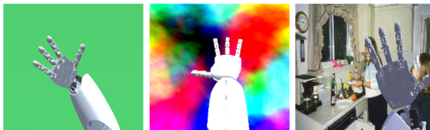
Figure 3.3: Solid color, Perlin noise and real backgrounds, from left to right, respectively.
