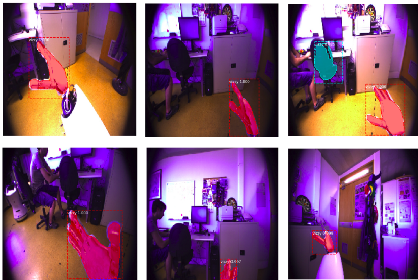
Figure 5.11: Visualization of the predicted masks, bounding boxes and class scores, for 6 images of the high clutter real validation set.
