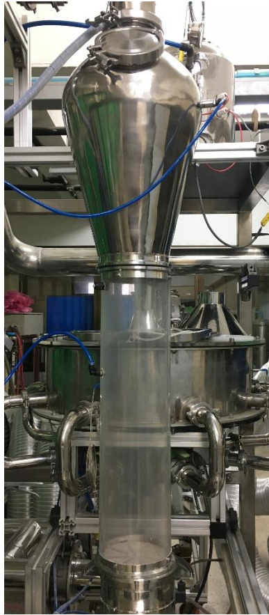
Figure 13- Pilot-scale fluidization unit available in the Faculty's laboratory
