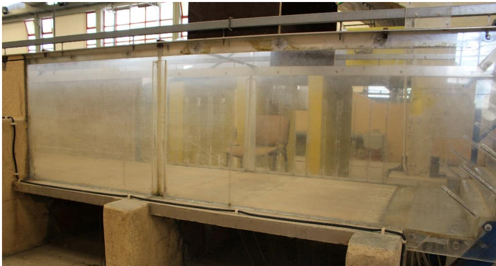
Figure 3.7: First half of the stilling basin made of acrylic glass
