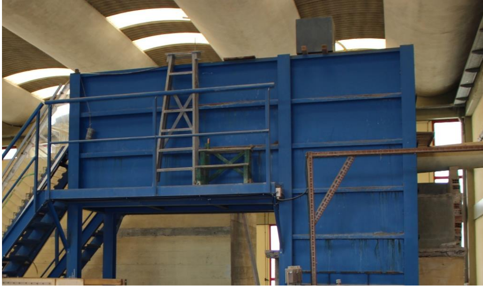
Figure 3.1: Upstream reservoir of the test assembly
