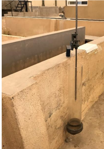
Figure 3.10: Hydrometer to measure depth and estimate discharge from the Bazin weir rating curve
