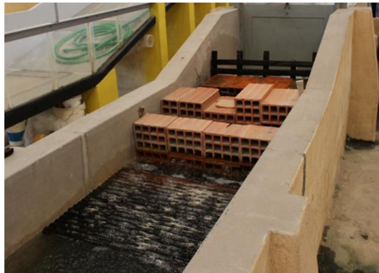
Figure 3.9: Flow control structures: Sluice gate (Left); Brick walls and wooden frame (Right)
