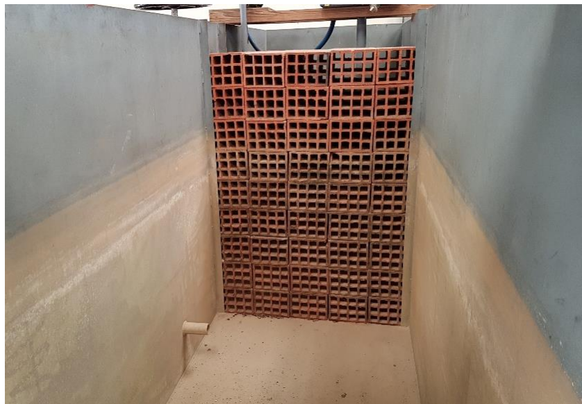
Figure 3.2: Brick wall in upstream reservoir
