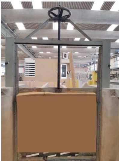
Figure 3.9: Flow control structures: Sluice gate (Left); Brick walls and wooden frame (Right)
