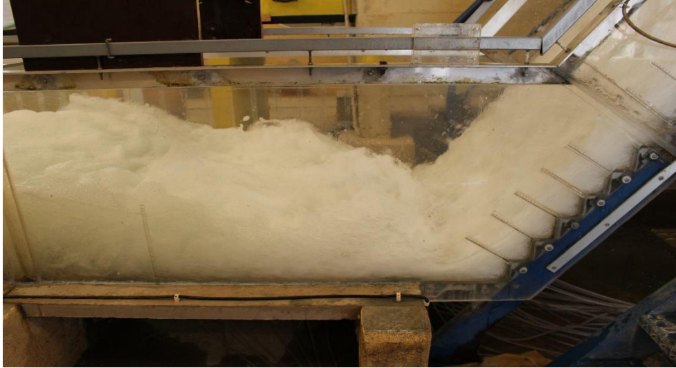
Figure 3.8: Visualization of a hydraulic jump through the clear acrylic walls of the stilling basin
