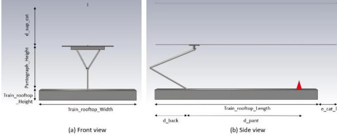
Figure 8. Rooftop/Pantograph/Catenary CST model
