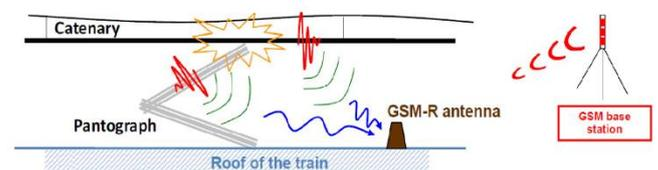
Figure 1. Pantograph and Catenary (from [13])
