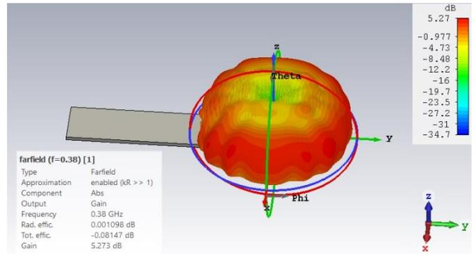
Figure 6. 3D farfield view at 380 MHz
