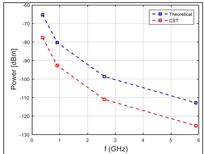
Figure 7. Harmonic's Interfering power
