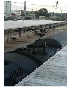
Figure 4. Pantograph and Catenary – Azambuja's station
