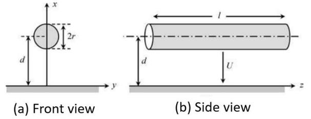
Figure 3. Cylindrical conductor above ground
