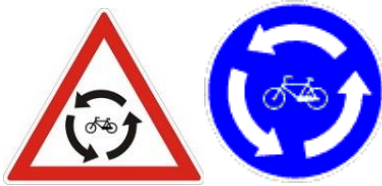
Figure 5 – B7b e D4b, signs for a bicycle lane with revolving circulation (adapted from Infraestruturas de Portugal and Diário da República, 1998).
