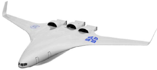
Figure 2.3: Cambridge-MIT Institute design using multiple fans driven by a single core engine [10]
