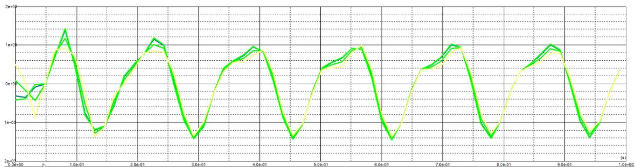
Figure 7 – Time history analysis – Velocity (mm/s) – Direction X: Max velocity ~1.4 mm/s
