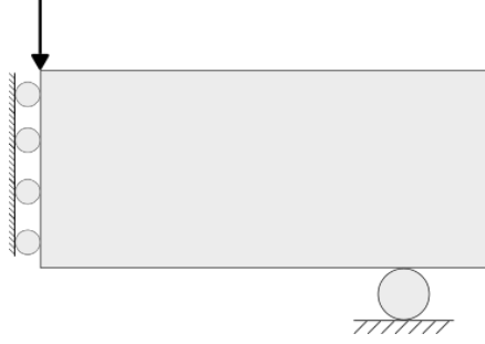
(a) MBB half-beam design space and loading conditions
