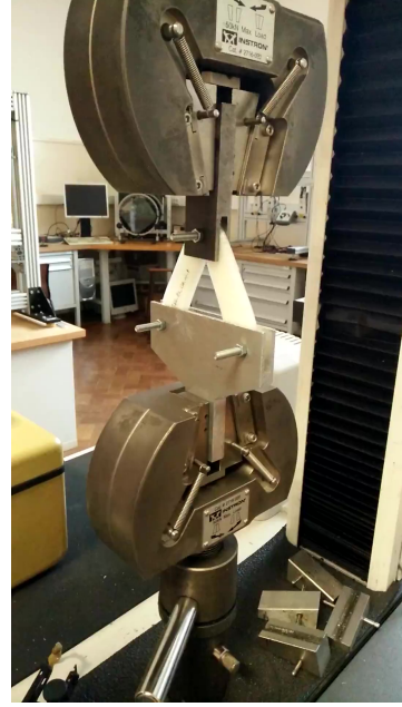
Figure 10: Experimental setup for the testing of the 3PT structures
