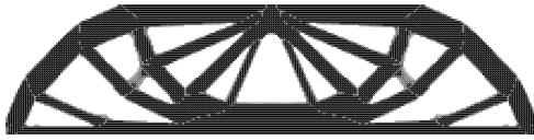
(a) Final optimal material and fiber angle distribution for the MBB_ORTHO optimization
