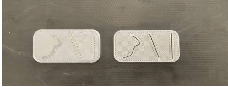
Figure 4.19: Side by side comparison of using the Expand thin features ON and OFF, respectively
