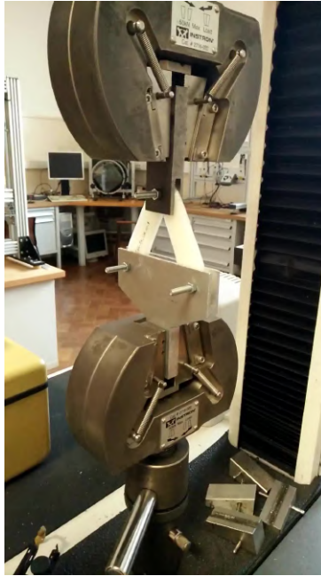
Figure 4.23: Experimental setup for the testing of the 3PT structures
