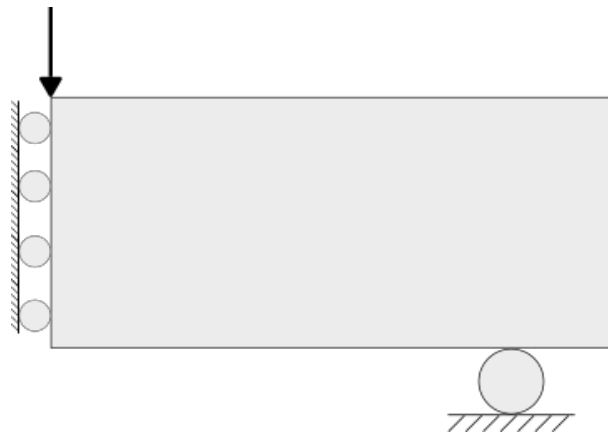
Figure 3.8: Loading and boundary conditions for one half of the MBB beam
