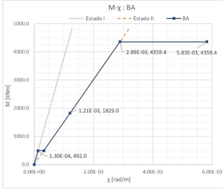
Figure 6.5- M- $\chi$  relation for the RC section.
