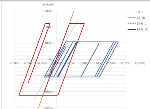
**Figure 6.11**-M- $\theta$  relation for the RC and RCFST sections after one time history analysis.
