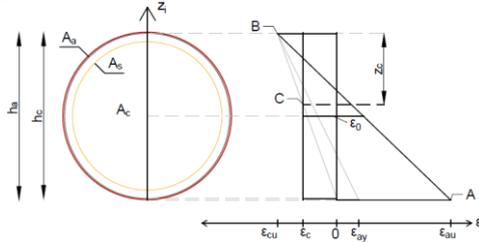
**Figure 5.7**-Admissible strain diagram for a RCFST section.
