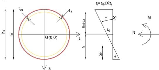
**Figure 5.8**-Reference axis definition for a RCFST section.
