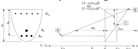
Figure 5.3-Admissible strain distribution [19].
