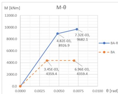
Figure 6.7- M- $\theta$  relation for the RC and RCFST sections.
