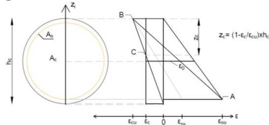
Figure 5.5-Admissible strain diagram for a RC section.
