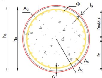
Figure 5.4-Generalized RCFST cross section.
