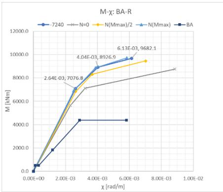
Figure 6.6- M- $\chi$  relation for the RC and RCFST sections.
