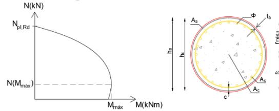
**Figure 5.9**-Bending moment-axial force (M-N) interaction curve for a generic RCFST section.
