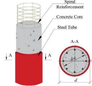
**Figure 3.2**-Layers of a RCFST [7].
