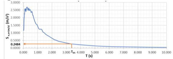
Figure 6.8- Average of the accelerations determined for a maximum acceleration of  $1m/s^2$ .
