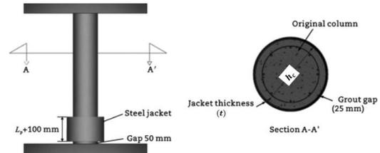
Figure 4.1-Retrofitted column, adapted from [18].
