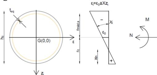
Figure 5.6-Reference axis definition for a RC section.
