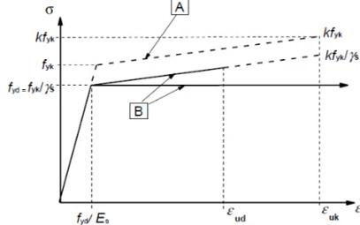
Figure 5.2-Stress-strain diagram for steel [19].
