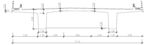
**Figure 6.3**-Midspan deck cross section.
