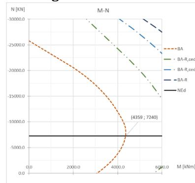
Figure 6.9- Maximum bending moment for a constant axial load,  $N_{Ed}$ .
