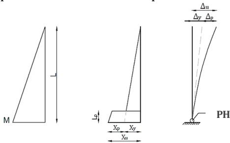
**Figure 2.3**-Plastic hinge concept, adapted from [2].
