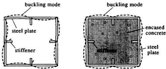
Figure 3.1-Buckling modes of steel and composite columns [12].
