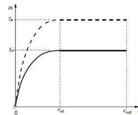
Figure 5.1-Parabola-rectangle diagram for concrete under compression [19].
