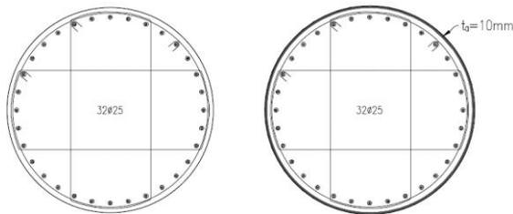
**Figure 6.2**-Original and reinforced cross section of the pier.
