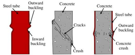
**Figure 3.1**-Collapse scheme of steel, RC and CFST sections, adapted from [6].
