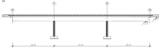
**Figure 6.1**-Side view of the viaduct.
