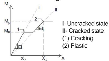
**Figure 5.10**-M- $\chi$  relation for a generic RC section.
