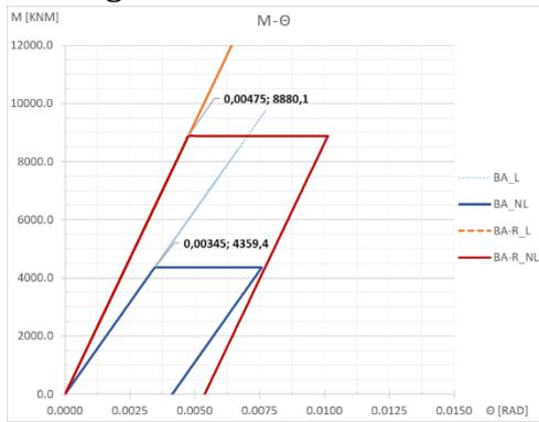
**Figure 6.10**-M- $\theta$  relation for the RC and RCFST sections.
