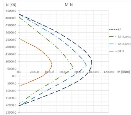
**Figure 6.4**-M-N interaction diagrams for the original and reinforced sections.
