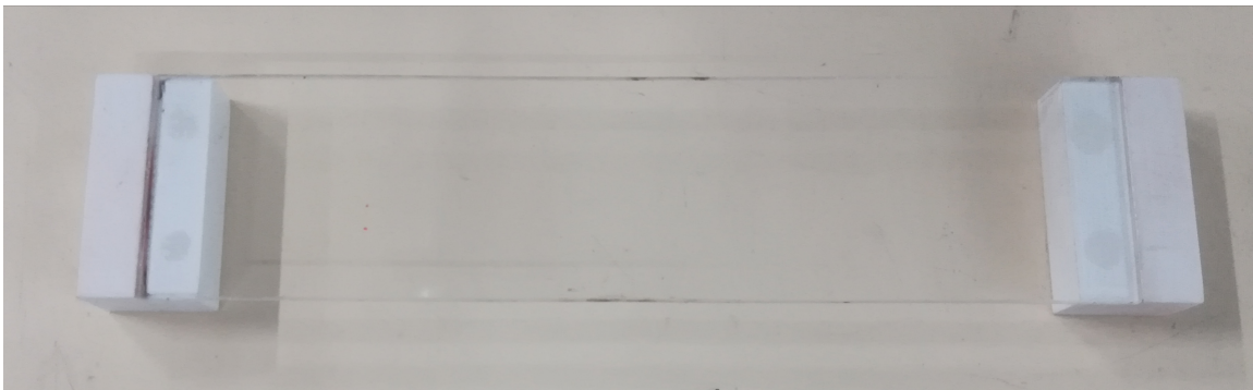
Figure 2.11: Image of the new outside entry wall for the experimental setup, with 3D printed parts and quartz glass.
