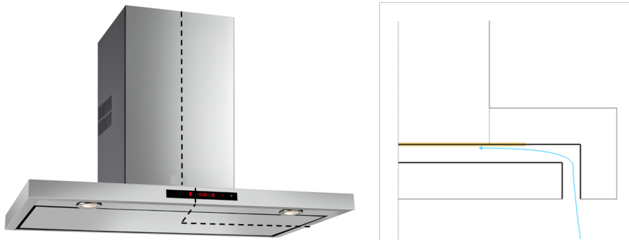
Figure 1.2: Cross-section representation of a perimetric exhaust (adapted from [3]).
