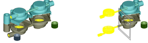
Figure 6: Line pressure represented on FEM model
