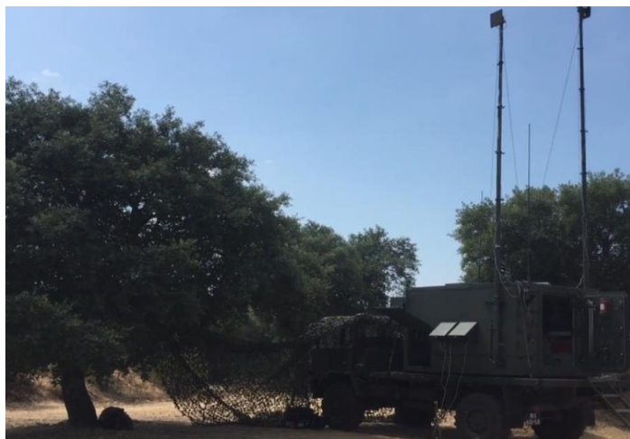
Figure 7 - Radio Access Point deployed in the “Leão 19”
