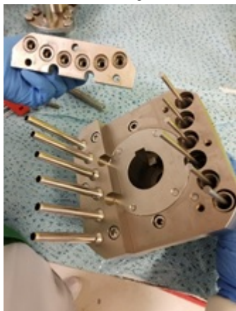
Figure 10: Zanasi dosing unit disassembled
