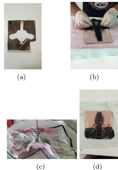
Figure 11: Component's manufacture: (a) Basalt fibre cutting procedure (second component) (b) Plies and insert placement on the mould (c) Vacuum assisted hand lay up process (d) Final component
