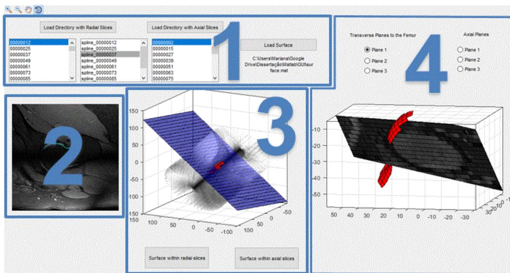
Figure 8 – GUI of the interactive application to evaluate the developed surface within the MRI sequences: (1) file region; (2) 2D plane; (3) viewing region of the 3D surface of the section to operate within radial or axial MRI sequence (4) viewing region of the 3D surface
