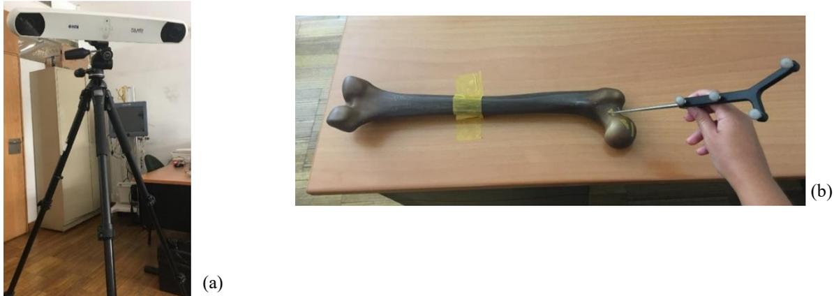
Figure 5 - Setup for registration process. NDI Polaris Spectra System (a) facing towards the realistic plastic femur and pointer (b).
