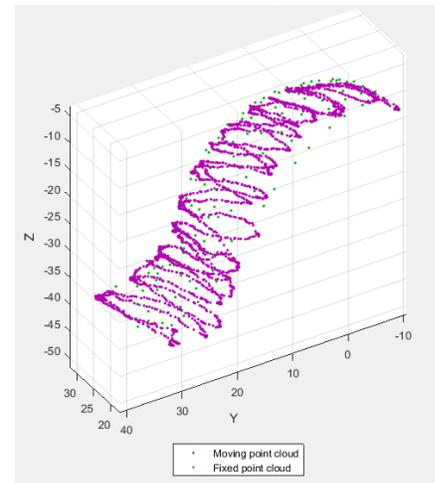
Figure 11 - Both point clouds after registration using ICP algorithm.
