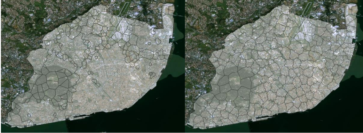
Figure 14 - Demand aggregation areas for Lisbon using the DBSCAN (left) and KM (right) methods.
