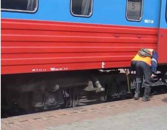
Figure 1 - Wheel-tapper testing a train's wheel by hammering (cf.: https://www.industryforum.co.uk )
