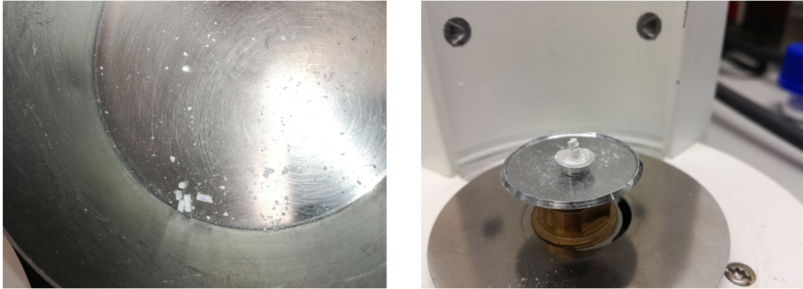
Figure 4.10: The figure on the left shows some powder slugs manually removed from the powder gun's tip when it jammed. Even after being dropped, some keep their cylindrical shape due to how compact they are. On the right, a slug that was pushed out of the gun during an air blast and stood vertically in the pan. It can compromise posterior dispensing and lid placement.
