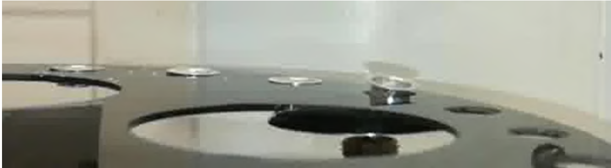
Figure 4.5: A detailed view of a protruding pan sliding onto the part placed in the balance. This is the method designed for sample weighing if using transport Module B.
