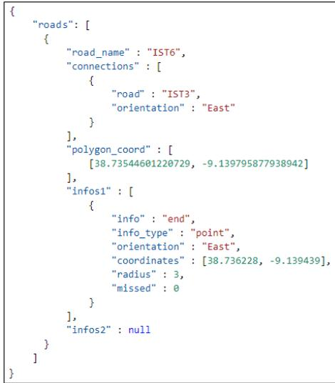
Figure 2: Illustrative example of a Graph Based Topological Map structure.
