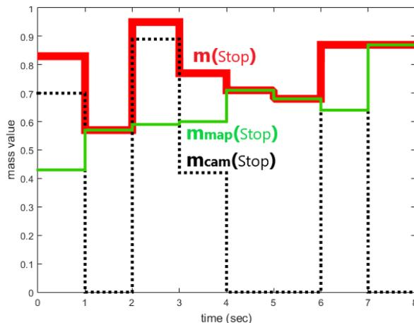
Figure 7: Fused mass  $m$ , in a situation where the TSRS output is unstable.
