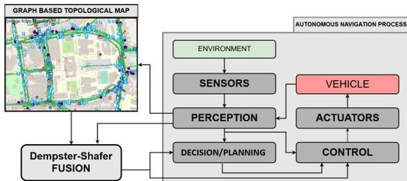
Figure 1: Interaction between the proposed system and the Autonomous Navigation Process.
