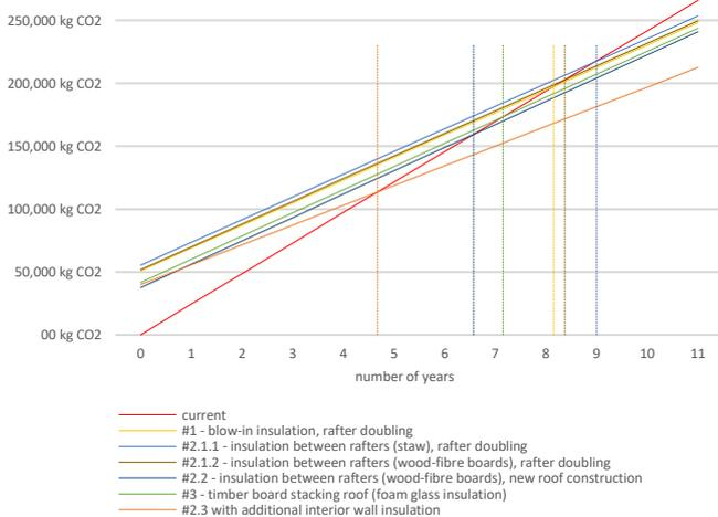
Figure 5: Overall CO<sub>2</sub> emissions for different design proposals
