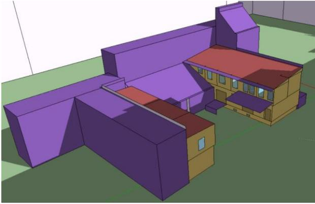
Figure 1: EnergyPlus model of the courtyard building
