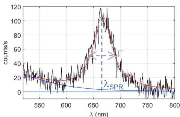
Figure 3: Example of the photoluminescence spectrum of a single rod and respective Lorentzian fitting to determine the peak wavelength  $\lambda_{SPR}$  (666 nm) and linewidth  $\Gamma$  (118 meV).
