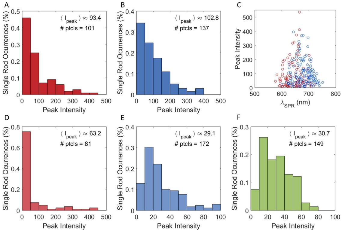
Figure 6: Histogram of Peak Intensity of single AuNRs in samples irradiated at 639 nm. Samples A – PVA Tip-1h; B – PVA FC-ON; C – PVA Tip-6h; D – PVA FC400-1h were irradiated at 0.04 kW/cm<sup>2</sup>. E – PVA LE was irradiated at 4 kW/cm<sup>2</sup>. F - Scatter graph of Peak Intensity relatively to surface plasmon resonance wavelength: PVA Tip-1h (○) and PVA FC-ON (◊).
