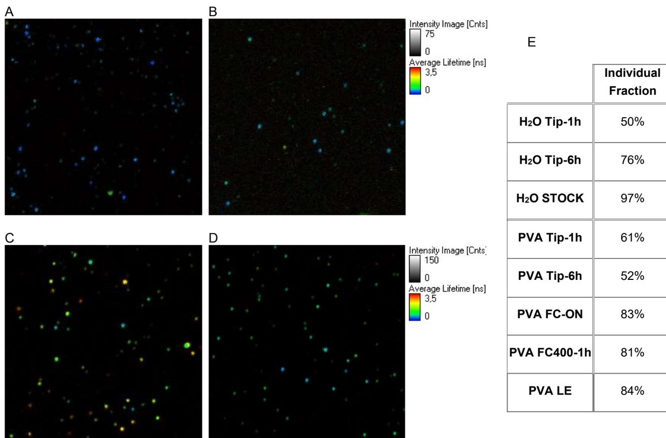
Figure 4: CFLM 40 x 40  $\mu\text{m}$  images at 639 nm laser irradiation. A – H<sub>2</sub>O Tip-1h at 0.04 kW/cm<sup>2</sup>; B - H<sub>2</sub>O stock at 20 kW/cm<sup>2</sup>; C – PVA Tip-1h at 0.04 kW/cm<sup>2</sup>; D – PVA FC-ON at 0.04 kW/cm<sup>2</sup>; E – Individual fraction – percentage of well-defined single AuNR recovered spectra for each sample.
