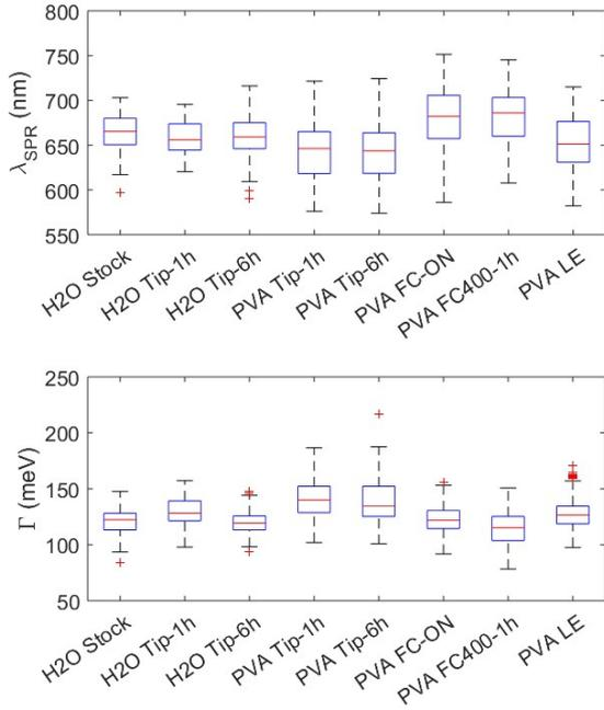
Figure 5: Boxplot of the surface plasmon resonance wavelength and FWHM obtained from Lorentzian fitting of single particle spectra.
