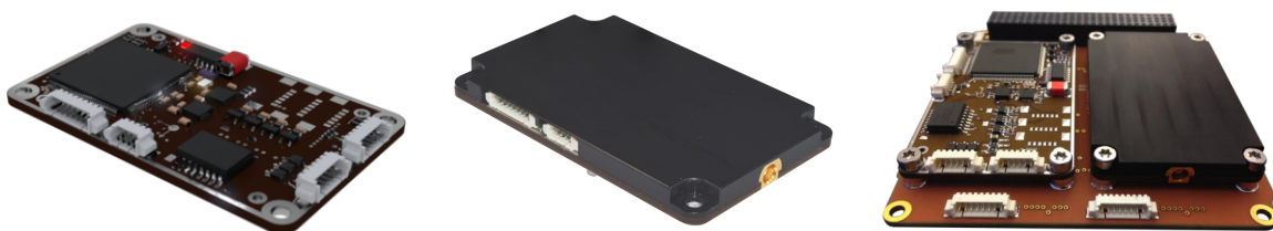
Figure 3.4: NanoMind A3200 (left), NanoCom AX100 (centre) and NanoDock DMC-3 (right) [adapted from [11]].
