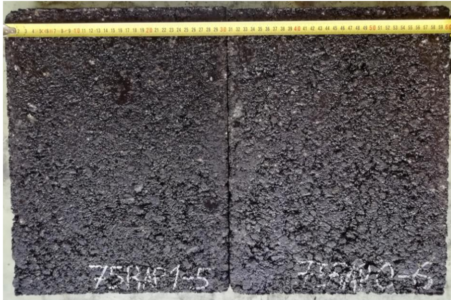
Figure 11: Surface texture comparison between 75% RAP (2 nd phase) (left) and 75% RAP (right)
