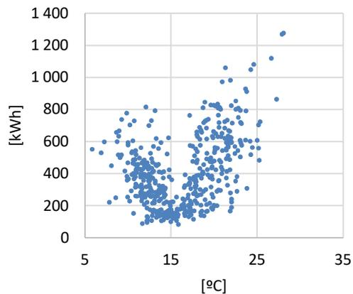
**Figure 4.1 HVAC consumption and outside temperature in 'Pavilhão Central'.**
