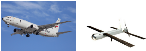
Figure 1.3: Left image: US Navy P-8A Poseidon. Right image: HAASW UTAS for the Navy P-8A Poseidon Maritime Patrol Jet [16]
