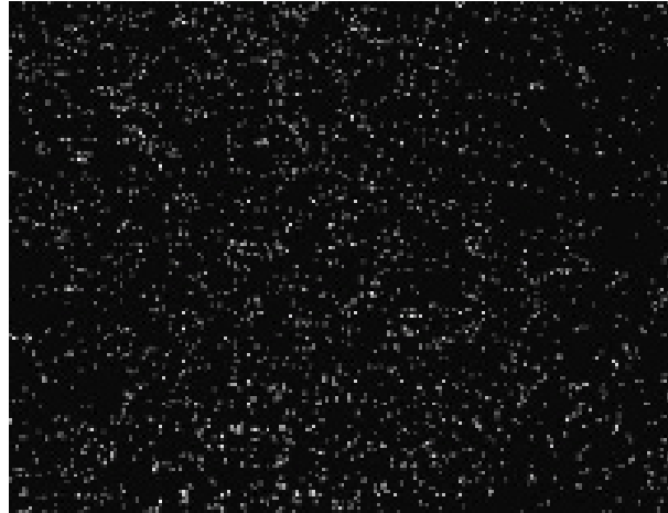
Figure 2.15: Seeding particles density standard.
