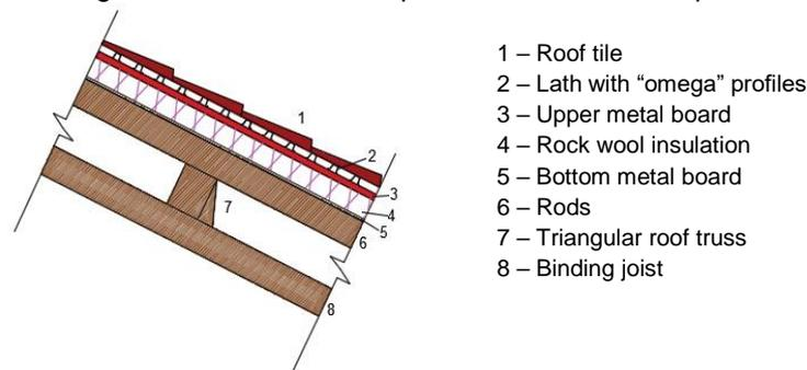
FIGURE 4 - CROSS SECTION OF THE ROOF (SOLUTION Nº2). DRAWING WITHOUT SCALE.
