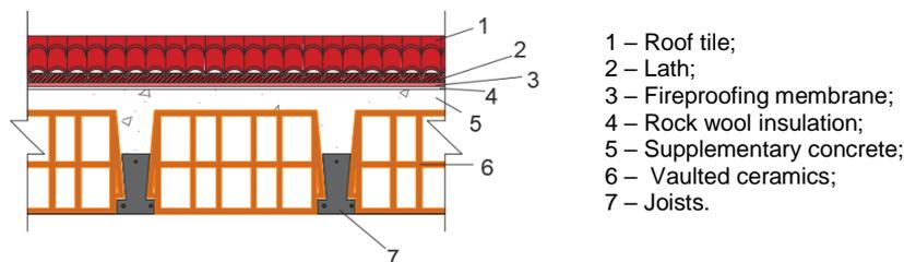
FIGURE 6 - CUT IN THE LONGITUDINAL DIRECTION OF THE SLOPING ROOF. DRAWING WITHOUT SCALE.
