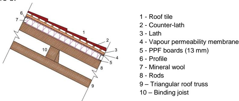
FIGURE 3 - CROSS SECTION OF THE ROOF (SOLUTION Nº1). DRAWING WITHOUT SCALE.
