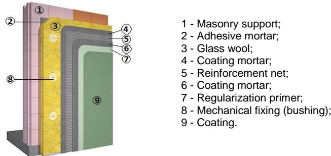
FIGURE 5 - EXTERIOR INSULATED WALL COMPONENTS (WEBER SOLUTION), ADAPTED FROM WEBER, 2018.
