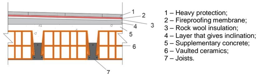
FIGURE 7 - CUT IN THE LONGITUDINAL DIRECTION OF THE TERRACE ROOF. DRAWING WITHOUT SCALE.
