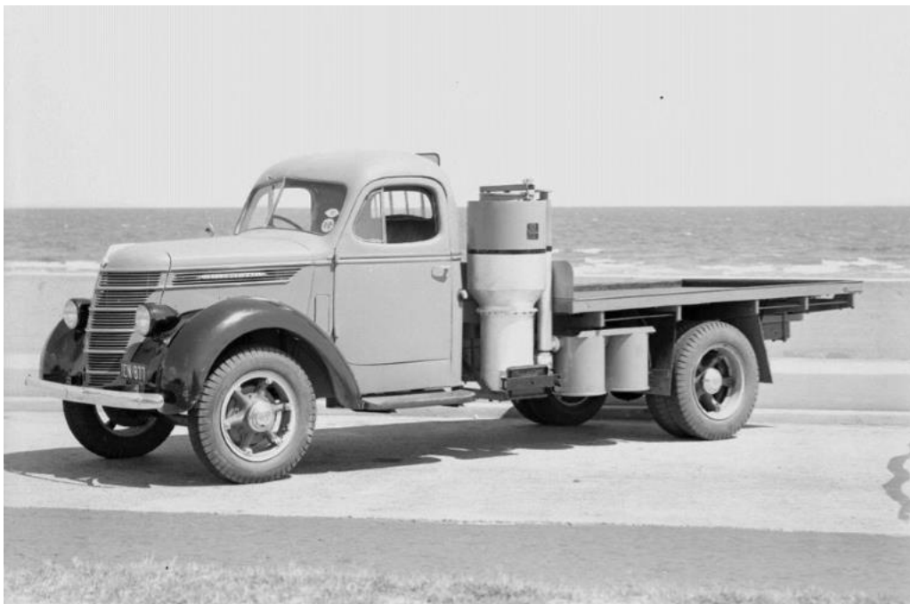
Fig. 18 Gasifier in motor vehicle [40]
