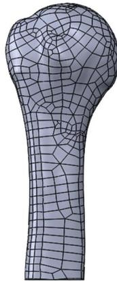
Figure 4-5 – Anterior view of the 3-D solid model of the proximal right humerus obtained using the software Solidworks®.
