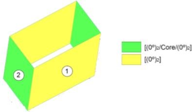
Figure 1: Optimized geometry and layup [1].
