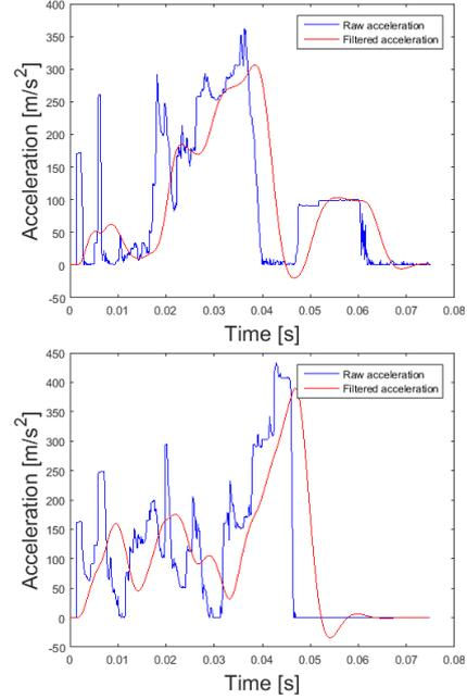
Figure 13: Acceleration curves for different corner radii -  $r=5$ mm (top) and  $r=25$ mm (bottom).
