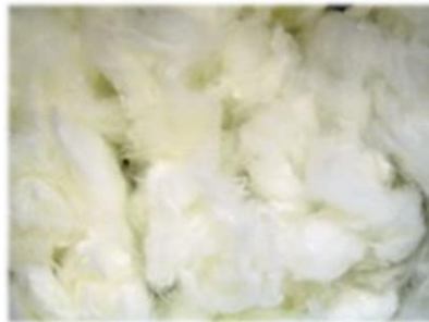
Figure 7. Acrylic fiber – staple
