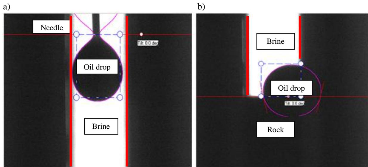
Figure 2. Interfacial tension, (a) and Contact angle, (b) calculation by Attension Theta software.
