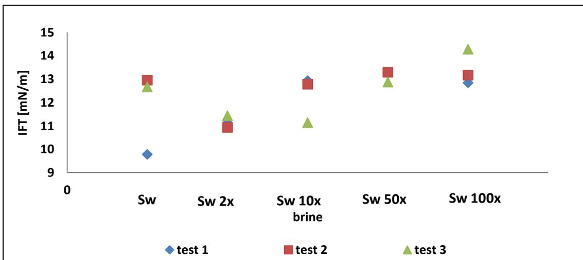
Figure 4. Values of IFT vs. dilutions considering the three tests.
