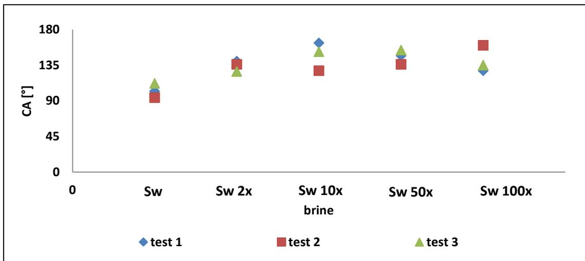
Figure 5. Values of CA vs. dilutions considering the three tests.
