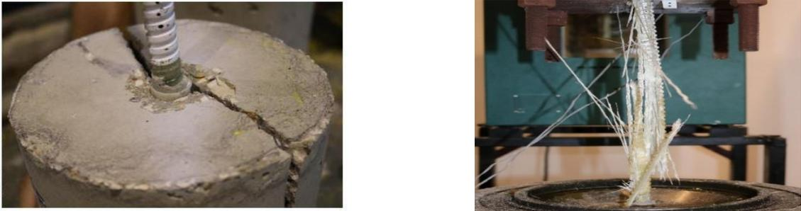
Figure 9 – Failure modes observed during the pull-out tests performed: (left) splitting failure in the straight rebars at 100 °C; (right) bent rebar at room temperature.
