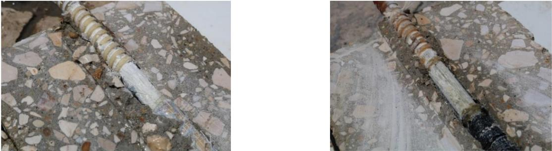
Figure 8 –(left) specimen tested at 140 °C; (right) specimen tested at 220 °C.
