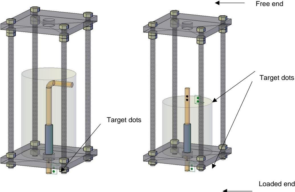
Figure 3 – Pull-out test setup used: (left) bent rebars; (right) straight rebars.
