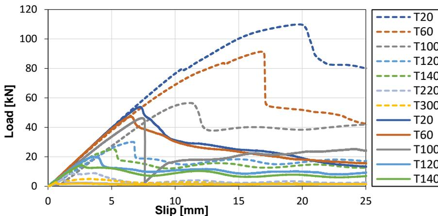
Figure 5 – Load-displacement average curves: (full line) straight rebars; (dashed line) bent rebars
