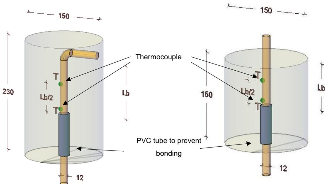
Figure 2 – Pull-out test specimens geometry and thermocouples placement: (left) bent rebars; (right) straight rebars), (dimensions in mm).
