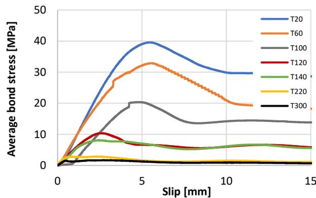
Figure 7 – Average bond stress vs. slip curves of the bent rebars.
