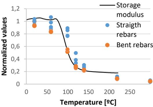
Figure 10 – Normalized values of the average bond strength and the storage modulus.
