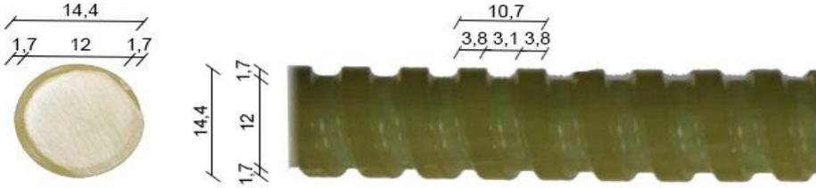
Figure 1 – GFRP rebar used in the present experiment (dimensions in [mm])
