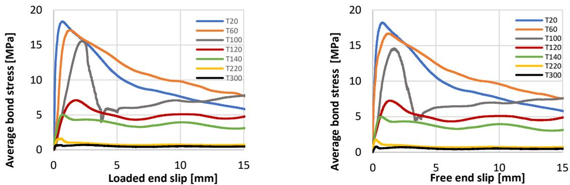
Figure 6 – Average bond stress vs. slip curves of the straight rebars: Loaded end slip(left); free end slip (right).
