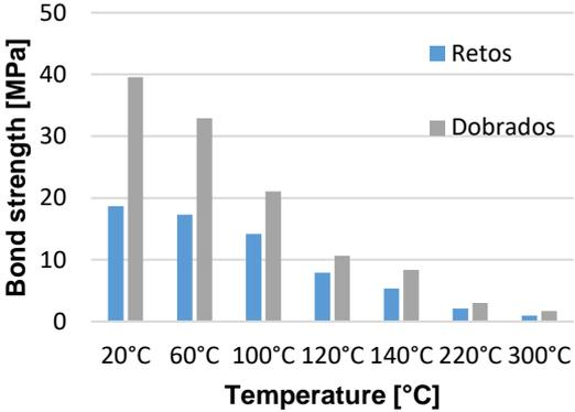
Figure 11 – Absolute values of the bond strength for both types of rebars.
