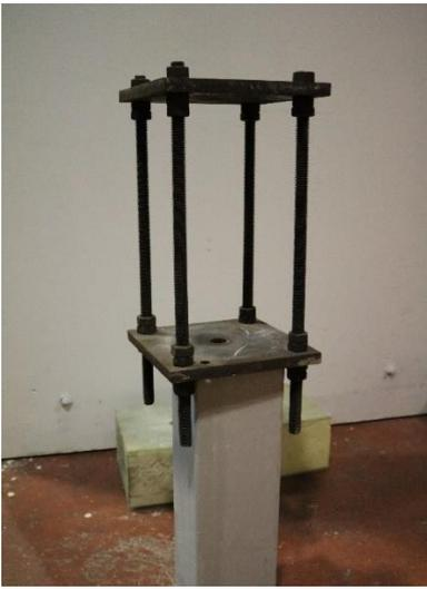
Figure 4 – Instron Universal testing machine (left); metal frame used in the pull-out tests (right).
