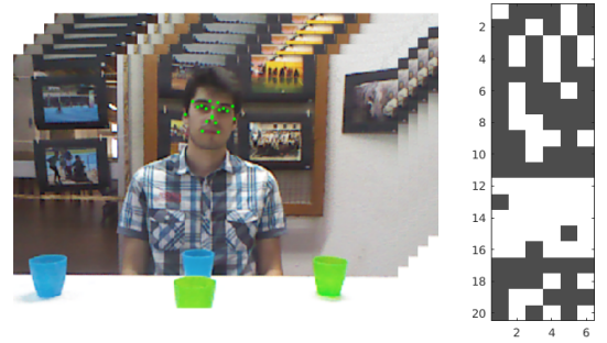
Fig. 2. Example of frame with points tracked (left), example of data matrix with correspondent missing (white) and known (grey) entries (right).
