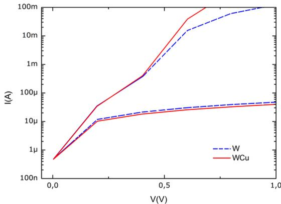
Figura 10: I-V characteristic semi-log curves of sample W in the dark before and after the Cu electrodeposition.
