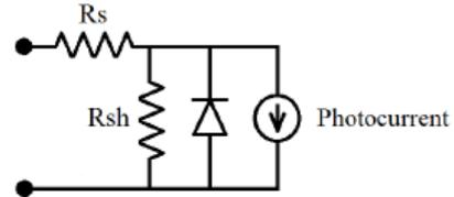
Figure 2: Equivalent circuit of a solar cell.
