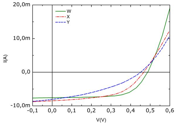
Figure 9: I-V characteristic curves W, X and Y under illumination (artificial light that simulates a *quasi* AM1.5 spectrum).
