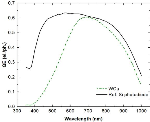
Figure 12: Quantum efficiency of sample W against a reference Si photodiode.
