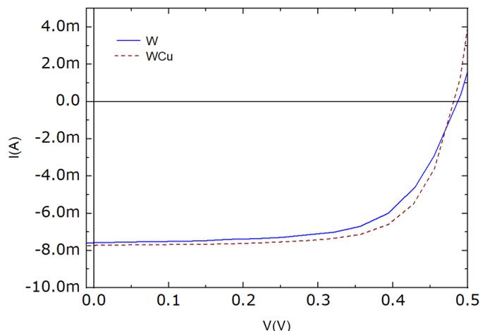
Figura 11: I-V characteristic curve of sample W under illumination (artificial light that simulates a *quasi* AM1.5 spectrum) before and after the Cu electrodeposition.
