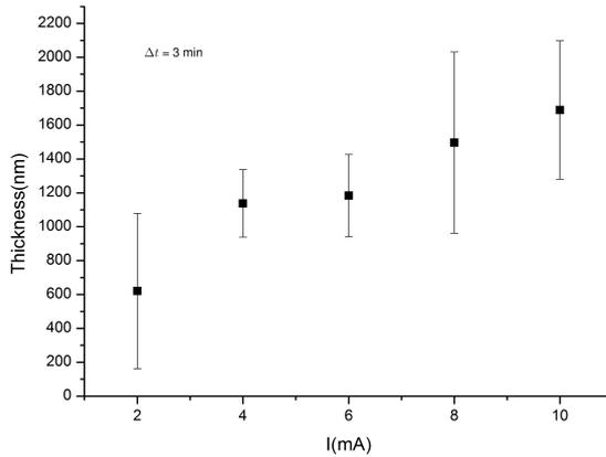
Figure 5: Electrodeposition study with constant  $\Delta t_{ED}$ : thickness as function of current for  $I = 2$  mA,  $I = 4$  mA,  $I = 6$  mA,  $I = 8$  mA and  $I = 10$  mA.
