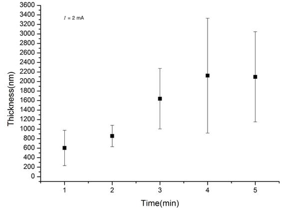
Figure 6: Electrodeposition study with constant  $I$ : thickness as function of  $\Delta t_{ED}$  for  $\Delta t_{ED} = 1$  min,  $\Delta t_{ED} = 2$  min,  $\Delta t_{ED} = 3$  min,  $\Delta t_{ED} = 4$  min and  $\Delta t_{ED} = 5$  min.
