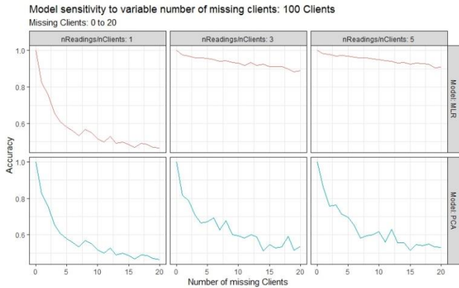
Fig. 13. Model sensitivity to variable number of missing clients for 20 runs and 100 clients.
