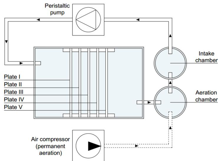
Figure 2 – Operating scheme of one of the reactors
