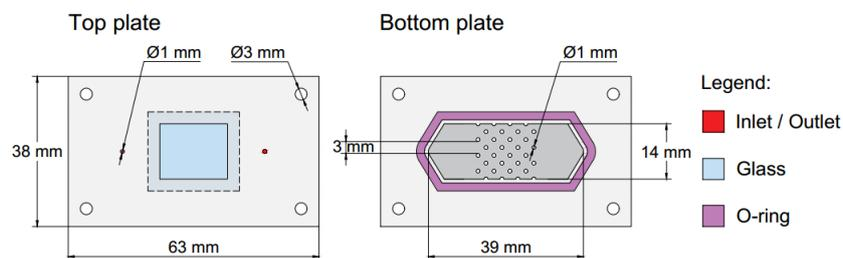
Figure 6 – 2D scheme of the microfluidic device
