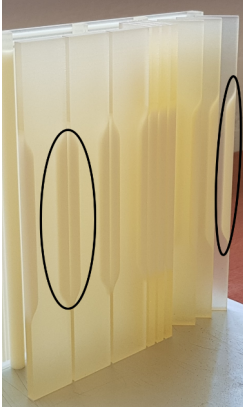
(b) Specimens after printing with support material.
