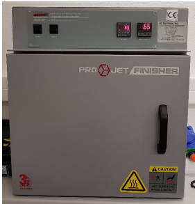
(b) 3D systems ProJet Finisher 1-B oven.
