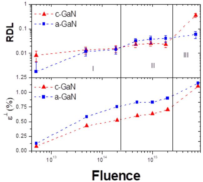
Figure 10 - RDL (relative defect level) and strain values for the depth window and regimes presented in Figure 5 as a function of the fluence.
