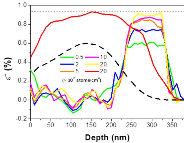
Figure 9 - Alternative RaDMax strain profiles for the fitting of the diffractograms of five a-GaN samples as a function of depth. The range of 380 nm for the depth axis corresponds to the maximum range of the argon atoms obtained from SRIM simulations. The SRIM vacancy-profile is included with arbitrary units. The red profile has been taken from Figure 8b for comparison.
