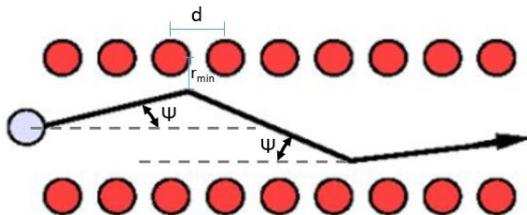
Figure 3 - Trajectory of the channeling of a particle.
