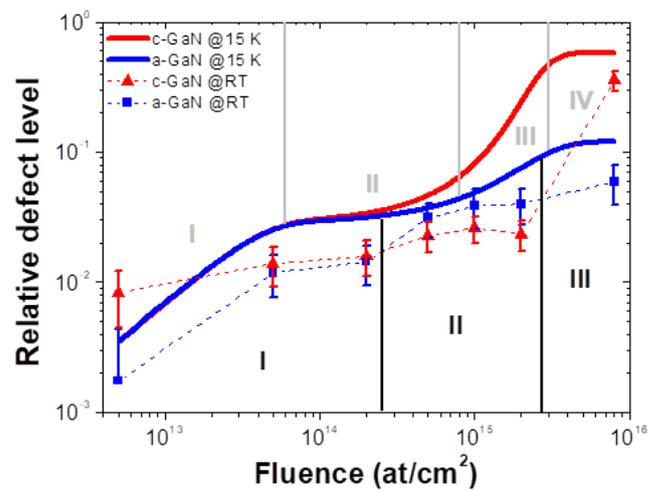
Figure 6 - Damage build-up curves. Simulated curves using Hecking's model from Lorenz et al. [12] at 15 K are shown for comparison with measured points (symbols and dashed lines) for both a-GaN and c-GaN.
