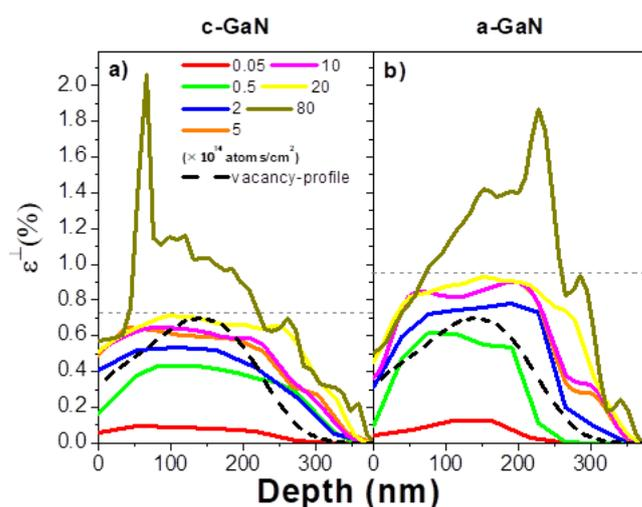
Figure 8 - Strain profiles derived using the RaDMaX code for a) c-GaN and b) a-GaN as a function of depth. The range of 380 nm for the depth axis corresponds to the maximum argon atom range obtained from SRIM simulations. The SRIM vacancy-profile is included for comparison with arbitrary units.
