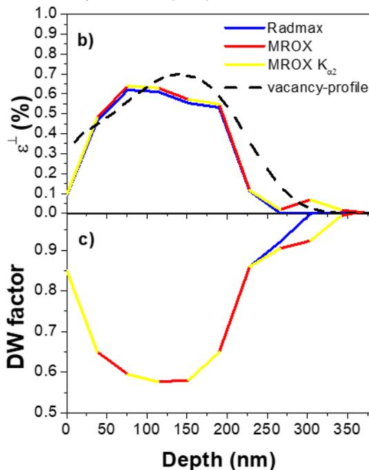
Figure 4 – Strain and DW factor profiles of an a-plane sample with an implanted fluence of  $5 \times 10^{13}$  atoms/cm<sup>2</sup>. Ten layers with the same thickness were defined, with a pre-defined Gaussian-like shape for strain profile (in red) and its "mirror" for DW. The damage depth is 380 nm, from SRIM.
