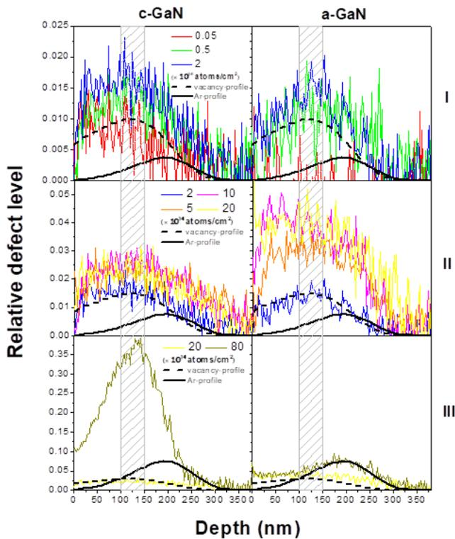
Figure 5 - Relative defect level profiles derived from the RBS/C spectra using a two-beam model for both planar orientations. Numbers on the right side of each row indicate the three different damage build-up stages. The distributions of argon and vacancies simulated using the code SRIM are included for comparison, with arbitrary units. The area between 100 and 150 nm is highlighted as it corresponds to the depth window used to plot the damage build-up (Figure 6).
