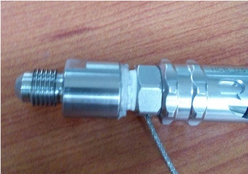
Figure A.8: Conic head necessary to maintain the air seal during the pressure measurement
