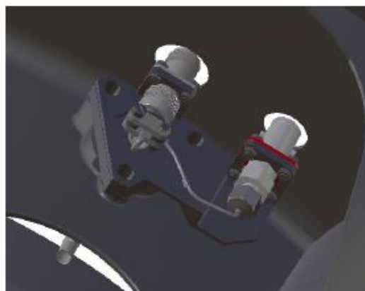
Figure 4.2: Positioning of the sensor on the CFM56-3 engine - Top view [27]
