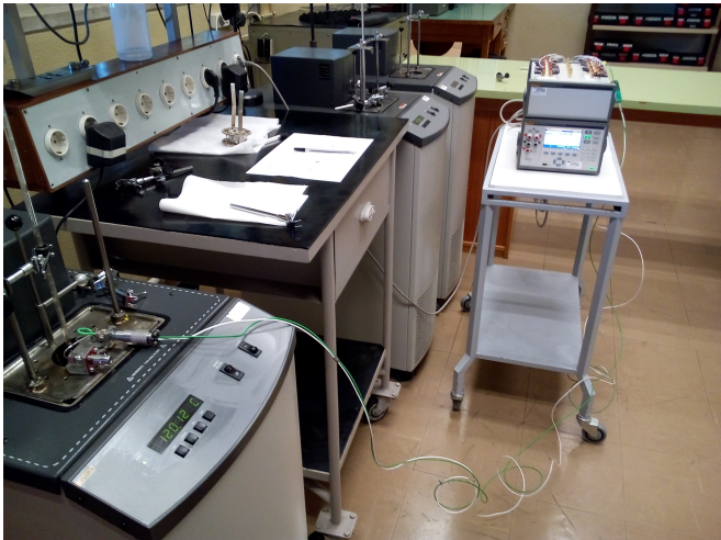
Figure 4.12: Second sensor temperature calibration test
