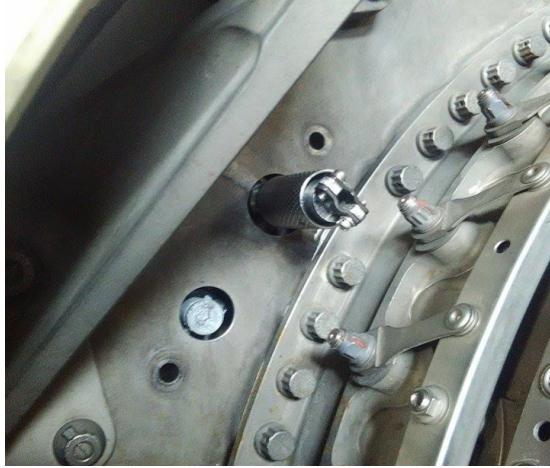
Figure 4.6: Successful test of 3D model with temperature plug attached
