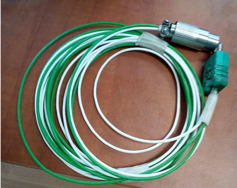
Figure A.12: Temperature connection from the sensor to the test bed
