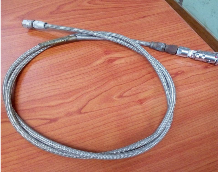
Figure A.11: Pressure connection from the sensor to the test bed
