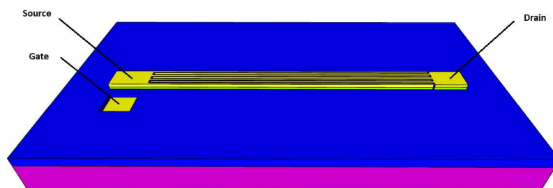
Figure 2 – Picture illustrating a back-gated CNT-FET for bio sensing application. In between the two interdigitated electrodes (Source and Drain) lies a network CNT's. The square pad is the gate electrode which connects to the Si layer below in order to apply the gate voltage through-out the channel. The FETs used in this study were provided by INESC-MN and have the same appearance as the one shown.
