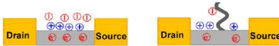
Figure 10 – How a dipole layer can be disrupted influencing the sensed field in the CNT-FET channel or near of the CNT/metal contacts, depending on the place of adsorption (31).
