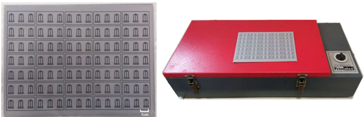
Figure 20 – Photoresist coated copper board with hard mask (Left). Primelec CI 2645 machine (Right).
